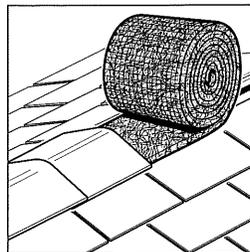
**STEP 4:** Install ridge cap shingles over top of vent using nails provided inside box. To ensure uniform look do not over drive nails. Ensure equal soffit ventilation.
