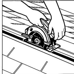
**STEP 2:** Cut opening 3/4" on each side of peak (for ridge board cut 1 3/4" on each side of ridge). Leave overhang uncut at each end of ridge. Do not cut roof truss or ridge board.
