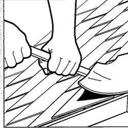
**STEP 1:** Remove ridge cap shingles along entire length of ridge.
