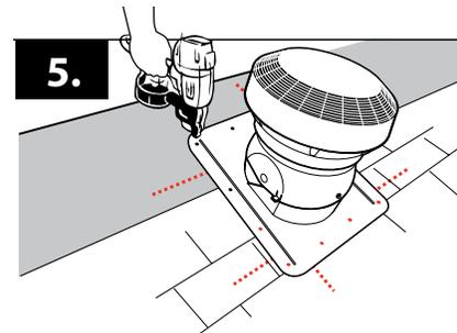
5. Position the roof vent over the cut opening in the roof. Center the vent by aligning edges of the vent throat with the chalk lines previously marked. Using the molded nail indicators, nail the top half of the vent securely into place.
