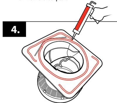
4. Using a 1/2 inch bead, apply a generous amount of construction sealant to the base of the vent.
