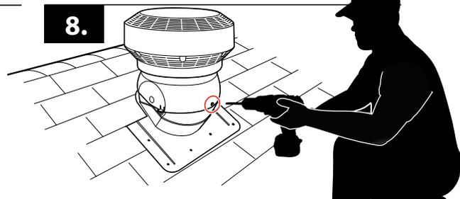
8. Using the molded in screw guide in front of vent, secure vent into position as shown with 1 screw supplied.
