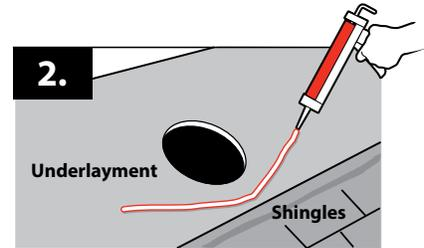
2. Using a 1/2 inch bead, apply a generous amount of construction sealant to the underlayment in front of hole before applying next shingle course.
