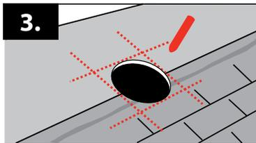
3. Install next shingle course over sealant bead and mark extended chalk lines to help position vent over opening in next step.
