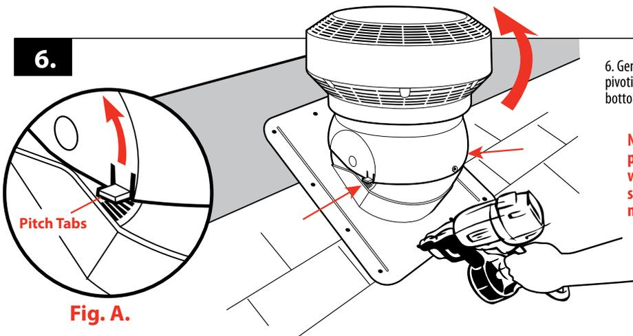
6. Gently lift the pitch calculating tabs (Fig A.), pivoting the top of the unit up to and nail the bottom half of the flange.
