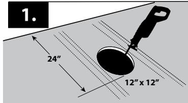
1. Apply underlayment on the sheathing and in the center of the rafters cut a 12" round hole. The edge of the hole should be at least 12" and no more than 24" from the roof peak.
